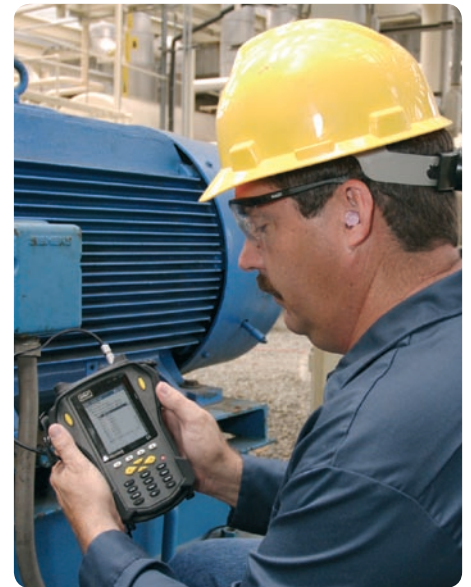
Recording vibration values using a SKF Microlog data collector
