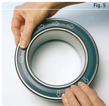
Inserting the seal in the outer ring
